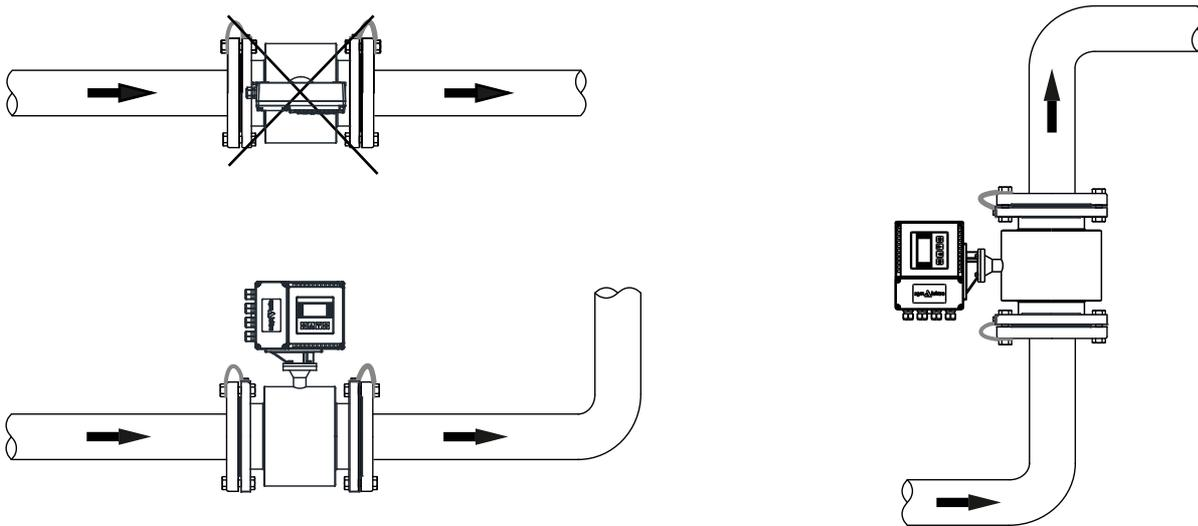
Installation in horizontal or vertical pipeline
