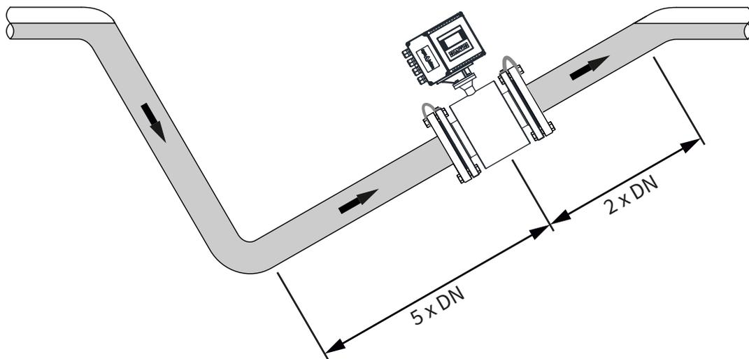
Installation in partially filled pipes
