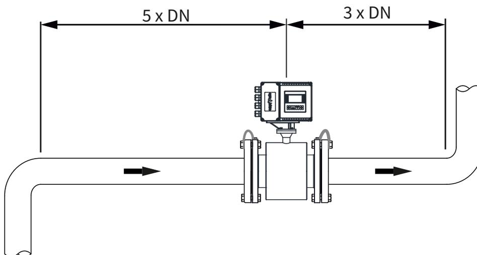
The electromagnetic flowmeter must be installed so that the pipe is always completely filled with fluid. In partially filled pipe case, the flowmeter must be installed with the siphon phenomenon, for which the pipe stretch where the meter is installed is kept always full.
