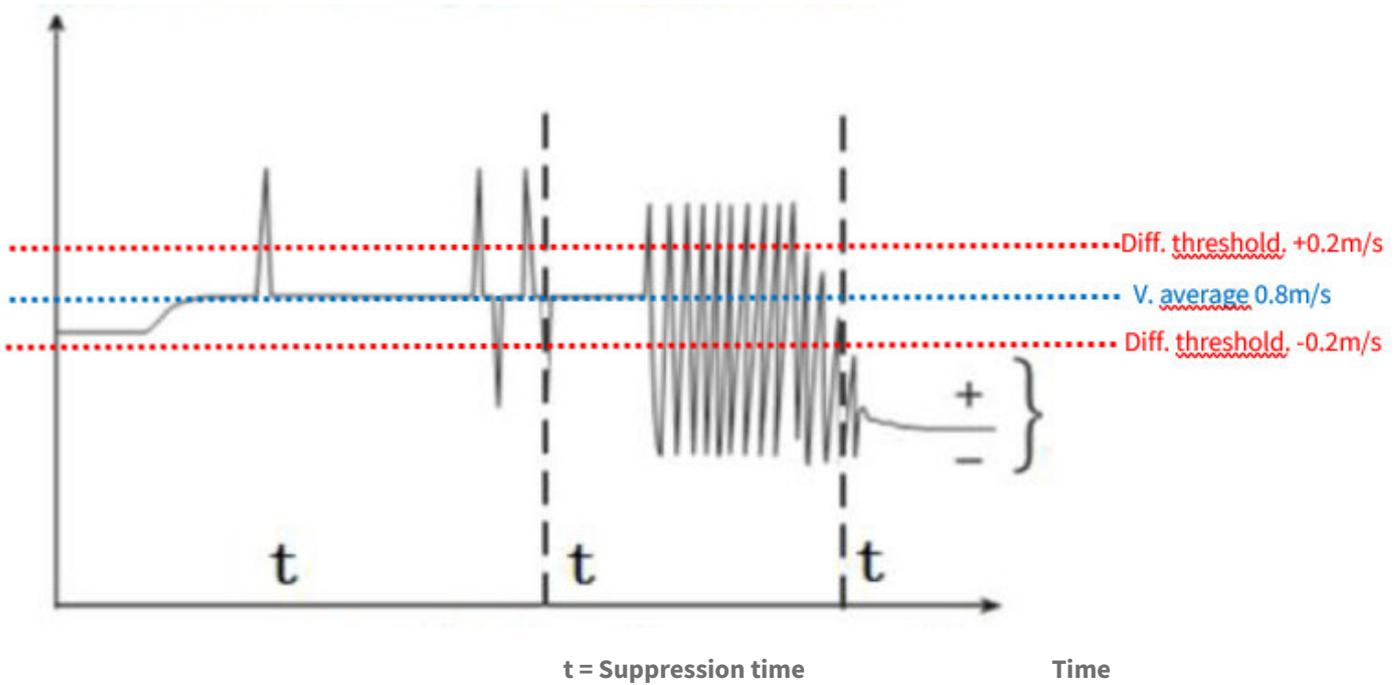
Resulting flow rate with Peak Limit Val filter. and Peak cut-off time
